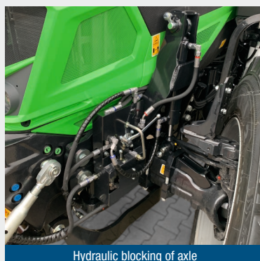
Hydraulic blocking of axle
