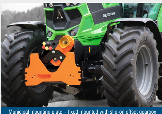
Municipal mounting plate – fixed mounted with slip-on offset gearbox
