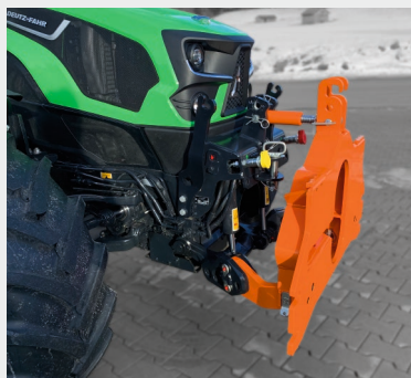
Mounting plate – simply fixed in front linkage
