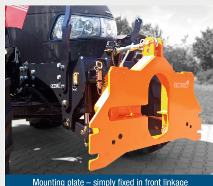
Mounting plate – simply fixed in front linkage
